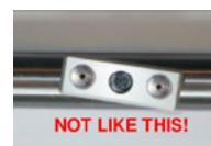
**3.6** CHECK: The sensor shall not move if you try to shake it slightly. The machined edges of the magnet-groove need to be in contact with the tie bar on the whole length.
