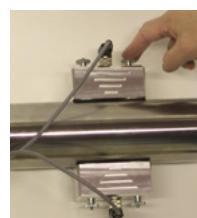
**3.5** If the magnet jumps off, then the spring force is too high. Loosen the adjustment nut 2 that the spring 3 is loosened (e.g. one rotation of the mounting nut counter-clockwise).
