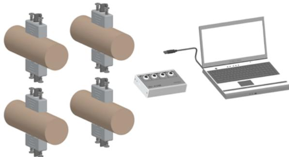
The 4-channel DU-4USB digital monitor box can only be operated in conjunction with a PC.
