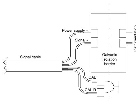
For models HMX2 and HWX2 with temperature measurement, the thermocouple circuit must be powered by means of galvanic isolation barriers with a maximum of 30V.
