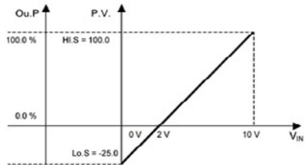
Since the 0...10V input range is reduced 80% above, the scale interval (HI.S – Lo.S) must be extended downward so that the useful interval (100.0 – 0.0) is 80% ( $100.0/125.0 = 0.8$ ).
