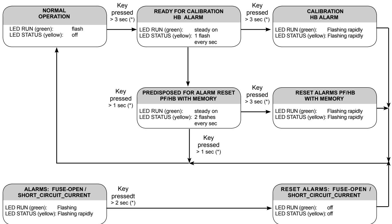
(\*) with key pressed, the state of the RUN and STATUS LEDs is steadily on; the LEDs switch off after 2/3 seconds to indicate switching to ready state
