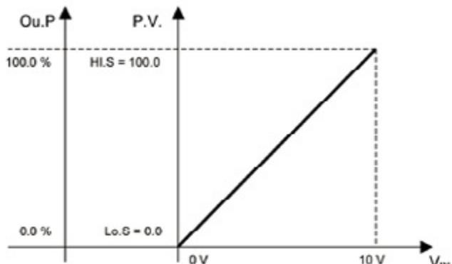
The default values (Lo.S = 0.0 and Hi.S = 100.0) can be changed to obtain the required scale of the PV in engineering value corresponding to the minimum and maximum of the physical input (V/mA).
