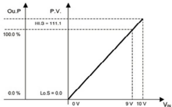
Since the 0...10V input range is reduced 90% below, the scale interval (HI.S – Lo.S) must be extended upward so that the useful interval (100.0 – 0.0) is 90% ( $100.0/111.1 = 0.9$ ).
