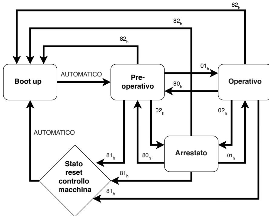
Every CANopen device contains an internal Network Management server that communicates with an external NMT master. One device in a network, generally the host, may act as the NMT master.
